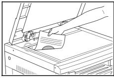
Set the copy original on the glass platen. Align the original so that the left rear corner is flush against the original size indicator.
