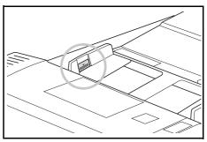
• When setting 11"  $\times$  17", 8  $_{1/2}$ "  $\times$  14", A3 or B4 originals open the Ejection Extension to prevent the originals from falling after ejection.
