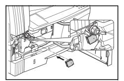
10 Pull the electrical charge section out as far as it will go and push it in after pulling it back and forth several times.
