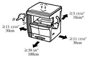
\* Additional space will be required when the Document Processor is to be installed.
