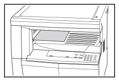
The finished copy will be ejected into the copy store section.
