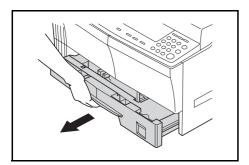
**5** If a sheet of paper is jammed inside, remove it carefully so as not to tear it.
