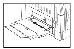
3 Use the Insert Guides to push the paper in until it reaches the point where it stops.
