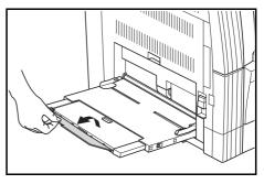
2 Adjust the Insert Guides to the width of the paper being set.
