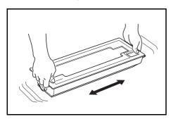
14 Turn Toner Container release lever (1) to the left and remove the Toner Container.
