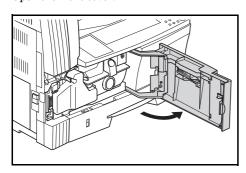
Push the Waste Toner Box holder to the left and remove the Waste Toner Box while pushing the holder.
