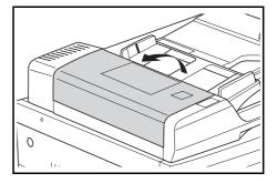
If an original is jammed inside, remove it carefully so as not to tear it.
