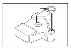
4 Set the new Toner Container in place, and turn Toner Container Release Lever (1) to the right.
