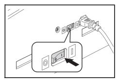
Turn ON (|) the Power Switch. The [Start] key will light up after warm up has been completed.
