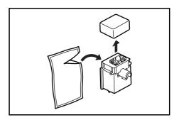
**9** Match the Grid Cleaner to the notch and install it in the copier main unit.
