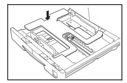
**3** Grasp the Width Size Adjustment tab and match the paper size to the Width Guide.
