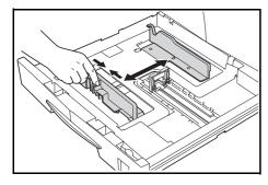
4 Grasp the Length Size Adjustment tab and match the paper size to the Length Guide.
