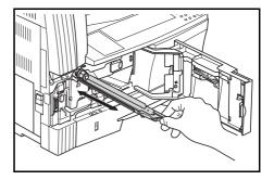
**11** Remove the Grid Cleaner and close the cap.
