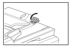
• In the case of Front and Back originals, the originals will be turned over so the originals will be temporarily ejected into the Ejection Tray. Do not handle the originals during this temporary ejection. Trying to pull an original out by force may cause a paper misfeed.
